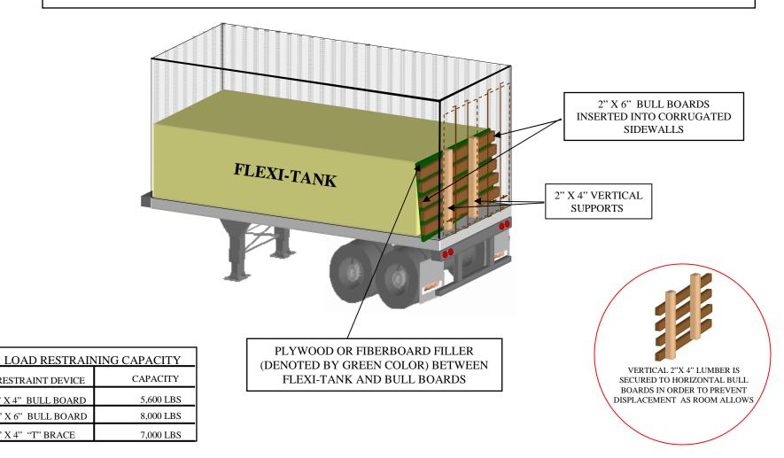
FLEXI-TANK DOORWAY SECUREMENT MUST NOT COME IN CONTACT WITH CONTAINERS DOORS
