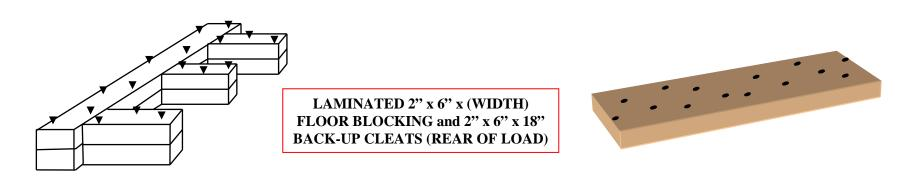
FLOOR BLOCKING SHOULD BE SECURELY NAILED TO THE TRAILER FLOOR AND MUST PENETRATE THE TRAILER FLOOR TO A DEPTH OF 1" OR MORE. THE NAILS SHOULD BE APPLIED IN A STAGGERED PATTERN, 4-6" APART.
