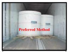
Loaded on End (Core Vertical)
